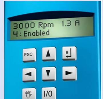
Display and keypad are integrated. So rapid diagnosis, status monitoring, direct parameter access and jogging (manual operation functions) are possible.
