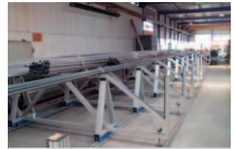
Long-item storage rack
